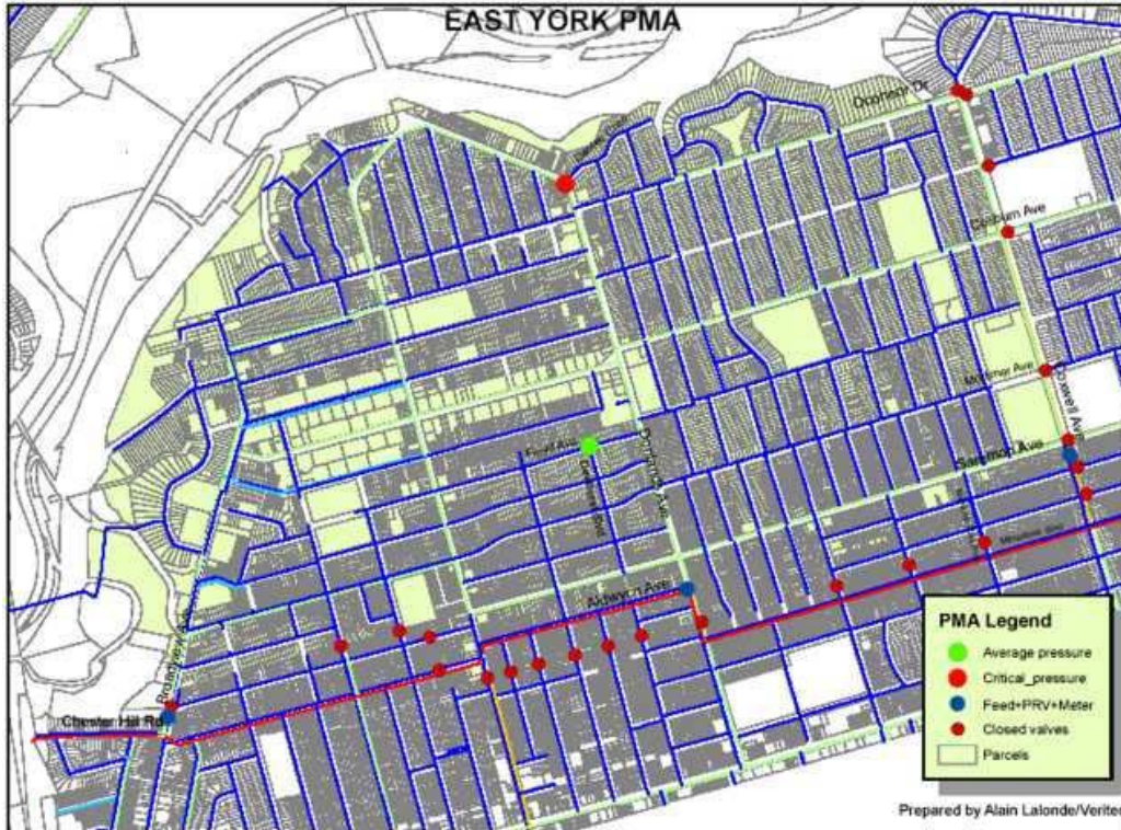
Figure 1 - East York Pressure Management Area Schematic
