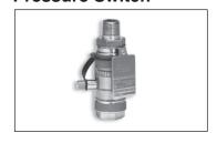
This durable, explosion proof Pressure Switch is used to signal that a deluge valve has opened. It can be specified on a new valve or easily retrofitted to an existing valve in the field.
