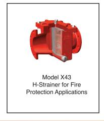
The X43 H-Style Strainer offers an effective means of removing unwanted particles or debris in pipeline flow. Ideal for mounting to directly to any Cla-Val Automatic Control Valve, the H-Strainers large flow area ensures a low pressure drop.
