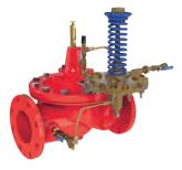
The 210 Series Altitude Valve is commonly used at reservoirs where water is withdrawn through a separate line or through a bypass line. The valve opens to refill the reservoir when the water reaches a point below the pre-set shut-off level. It is available in a variety of configurations including those designed for one-way flow and combination altitude and back pressure control.
