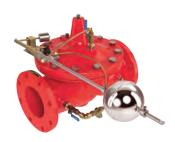
The 124 Series Float Valve provides an effective means of controlling the liquid level in fire water reserve tanks, opening or closing when the liquid level reaches its pre-set low and high points.
