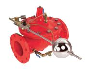
The highly accurate 129 Series Float Valve maintains a consistent level in large diameter fire water storage tanks and reservoirs by admitting flow into the tank in direct proportion to flow out of the tank.
