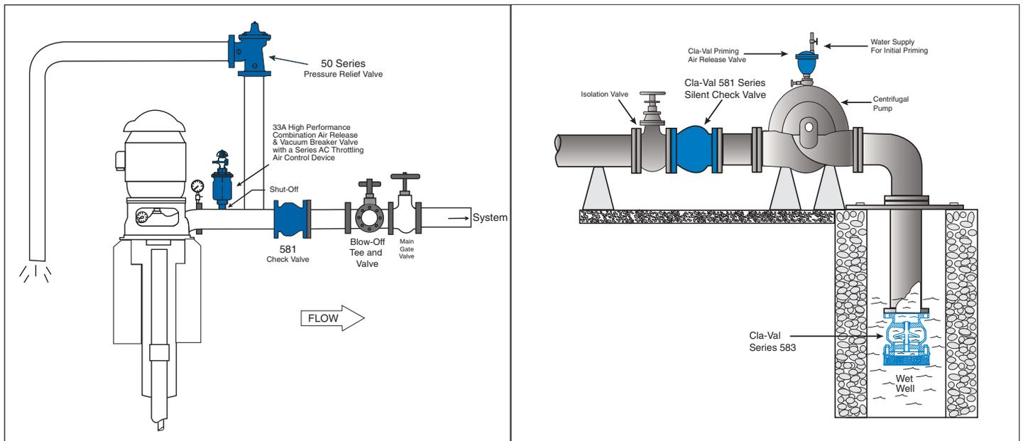
Cla-Val 581 Series Silent Globe Check Valves are used anywhere a quick, quiet closure is desired and in the majority of pump applications, including the following;
