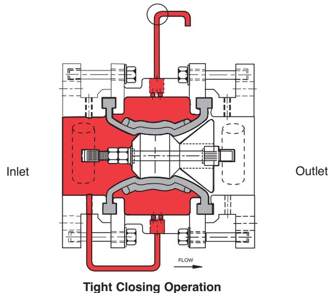
Water pressure from valve inlet is applied to the control chamber. Valve closes bubble tight.
