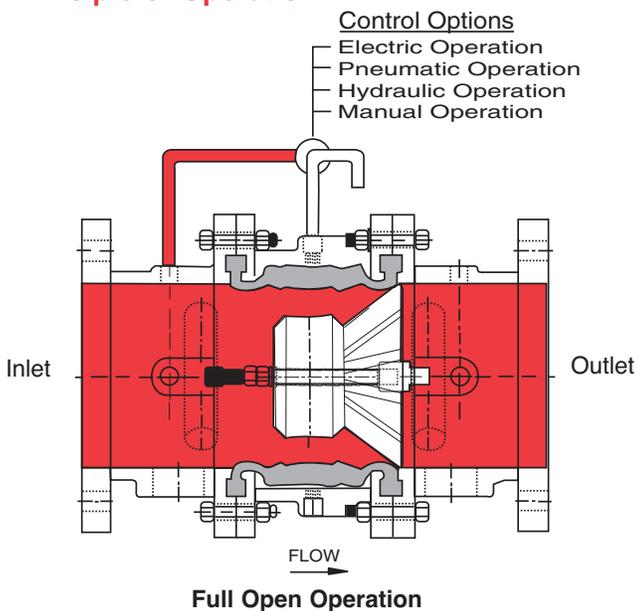
When pressure in control chamber is relieved, the valve is open.
