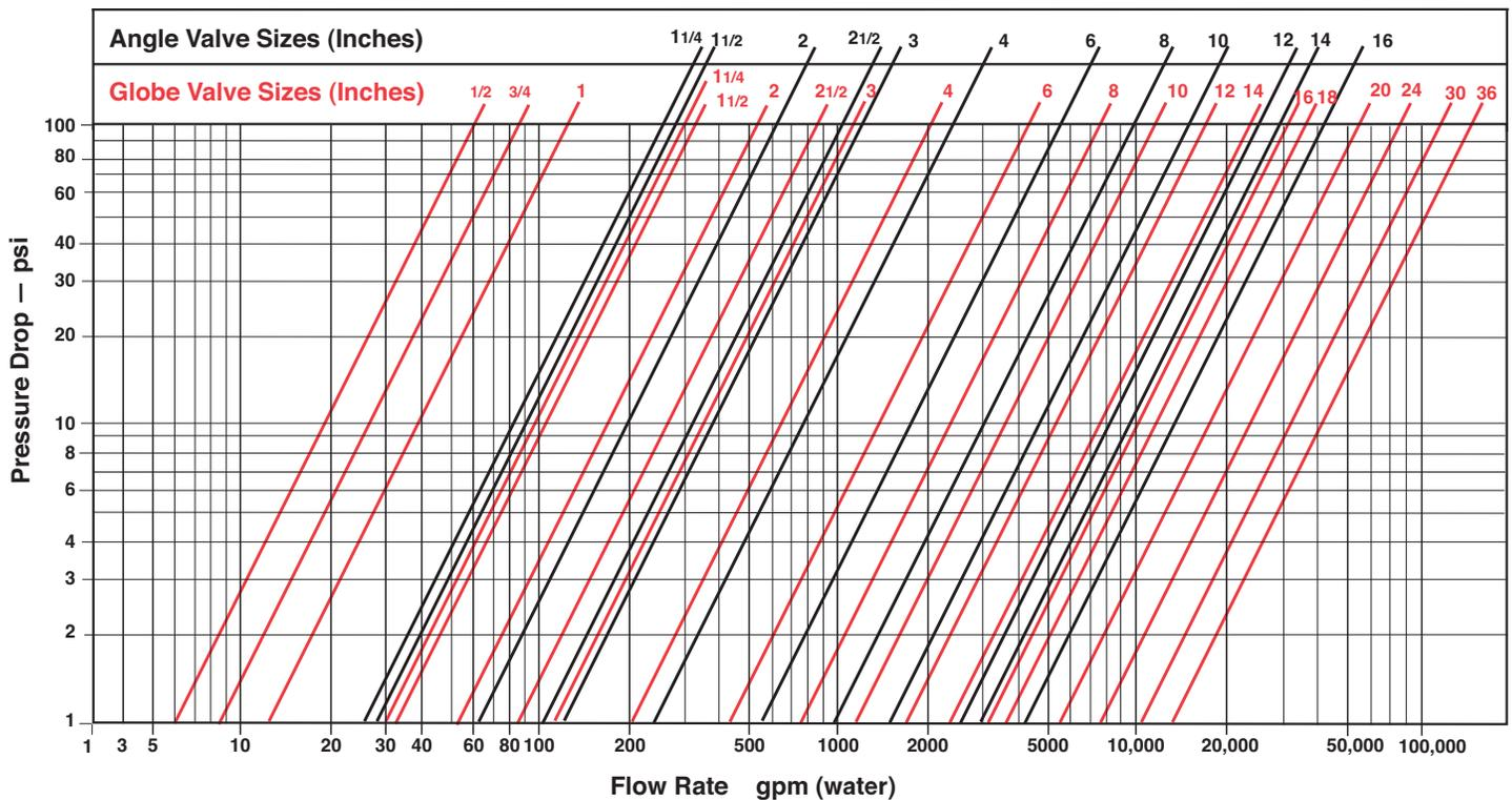
**NOTE:** The flow rate vs. head loss data presented here is based on a fully open valve condition. The maximum recommended velocity is 20 ft./sec.
