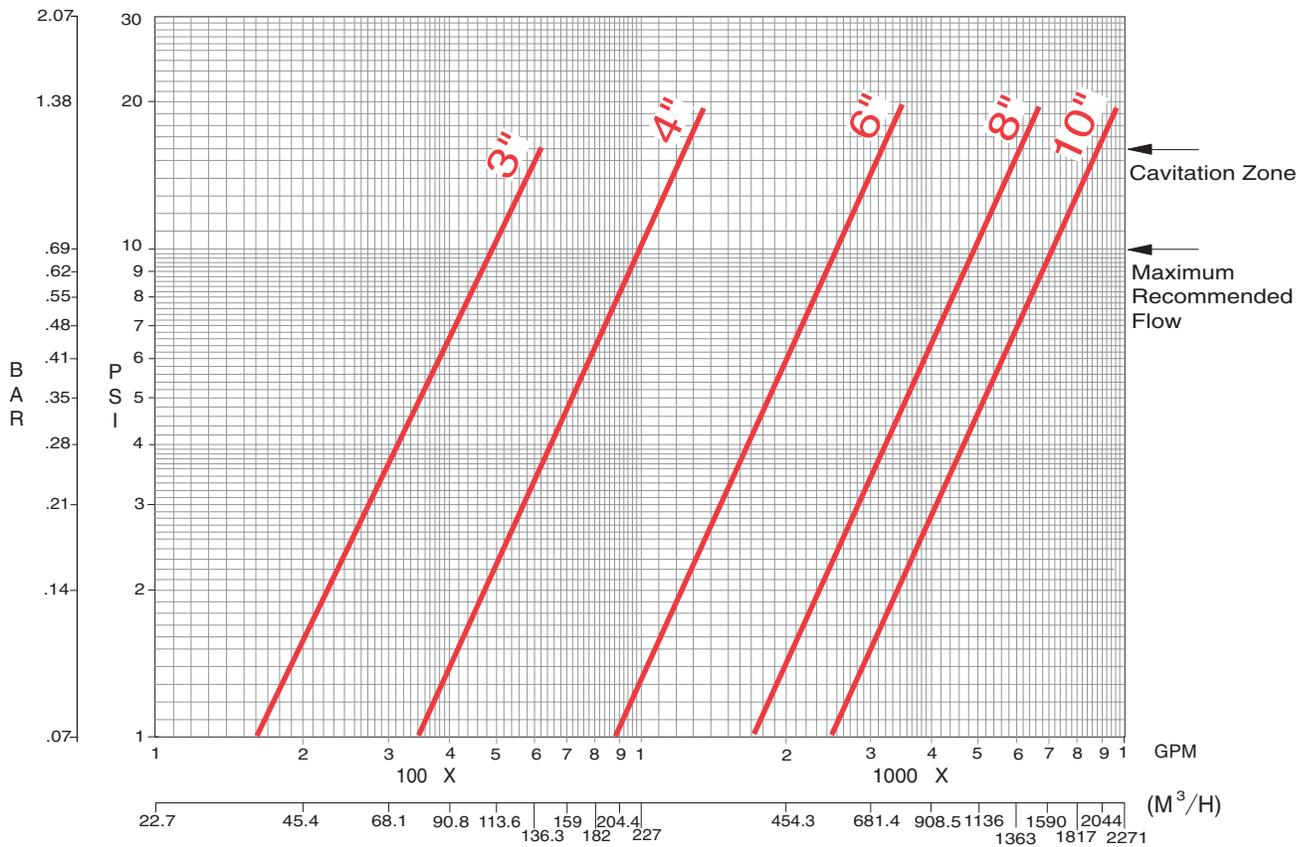
**NOTE:** The flow rate vs. head loss data presented here is based on a fully open valve condition. The maximum recommended velocity is 20 ft./sec.
