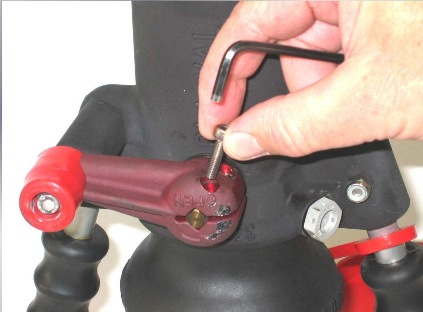
***Just loosen the inner screw – do not remove***
