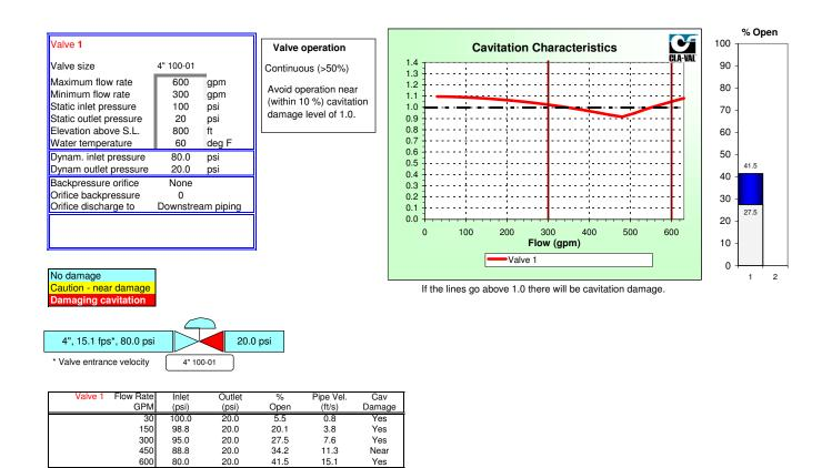
Now that we know there will be cavitation damage, what can we do about it? One method of combating cavitation damage is to add back pressure to the valve.
