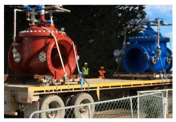
In 2013 after 7 years of continuous duty the first valve was taken out of service for inspection. A 16" (400 mm) Reducing valve and a 6" (150 mm) Reducing bypass valve.
