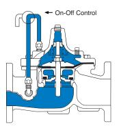
**Tight Closing Operation** When pressure from the valve inlet is applied to the cover chamber, the valve closes drip-tight.
