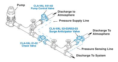
Install Model 661-02 valve as shown. Use a minimum of 12mm tubing to connect operating pressure connection of the valve to the system side of check valve. Flexible conduit should be used for electrical connections to the solenoid control and the limit switch assembly. A Model 52-02 or 652-03 Surge Anticipator is recommended for power failure and surge protection.
