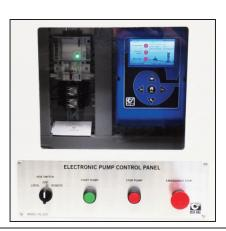
The Cla-Val PC-22D provides control of the pump and pump control valve, preventing surges in the system when the pump starts or stops. It consists of a pre-wired electrical control panel employing a programmable valve controller to sequence the pump and pump control valve during all modes of operation. Provides added protection to the pumping system from damage caused by mechanical, hydraulic or power failure.
