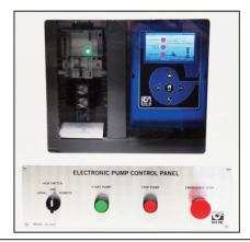
The Cla-Val PC-22D provides control of the pump and pump control valve, preventing surges in the system when the pump starts or stops. It consists of a pre-wired electrical control panel employing a programmable valve controller to sequence the pump and pump control valve during all modes of operation. Provides added protection to the pumping system from damage caused by mechanical, hydraulic or power failure.
