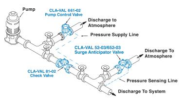
Install Model 661-02 valve as shown. Use a minimum of 12mm tubing to connect operating pressure connection of the valve to the system side of check valve. Flexible conduit should be used for electrical connections to the solenoid control and the limit switch assembly. A Model 52-02 or 652-03 Surge Anticipator is recommended for power failure and surge protection.
