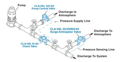
Install Model 661-02 valve as shown. Use a minimum of 1/2" tubing to connect operating pressure connection of the valve to the system side of check valve. Flexible conduit should be used for electrical connections to the solenoid control and the limit switch assembly. A Model 52-02 or 652-03 Surge Anticipator is recommended for power failure and surge protection.
