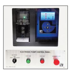
The Cla-Val PC-22D provides control of the pump and pump control valve, preventing surges in the system when the pump starts or stops. It consists of a pre-wired electrical control panel employing a programmable valve controller to sequence the pump and pump control valve during all modes of operation. Provides added protection to the pumping system from damage caused by mechanical, hydraulic or power failure.
