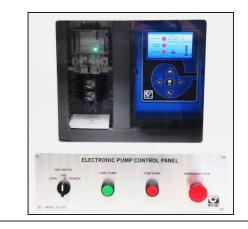
The Cla-Val PC-22D provides control of the pump and pump control valve, preventing surges in the system when the pump starts or stops. It consists of a pre-wired electrical control panel employing a programmable valve controller to sequence the pump and pump control valve during all modes of operation. Provides added protection to the pumping system from damage caused by mechanical, hydraulic or power failure.
