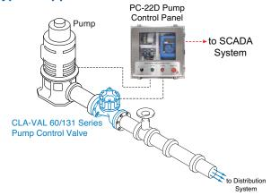
To minimize "in field wiring" the PC-22D is manufactured for most common pump control applications. The installation above shows the PC-22D being used with a Cla-Val Electronic Pump Control Valve.
