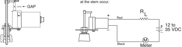
Coupler gap is set with valve in fully closed position. This establishes the minimum mechanical position for 4 mA output.
