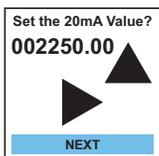
Use arrow keys to set 20mA Full Scale Output. Match 20mA value to customer display and/or SCADA. Select **NEXT** to continue.
