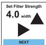
Default Filter is 4.00. Use arrow keys to increase or decrease filtering of 4-20mA signal. The higher the average filter strength, the longer the averaging time. Select **NEXT** to continue.
