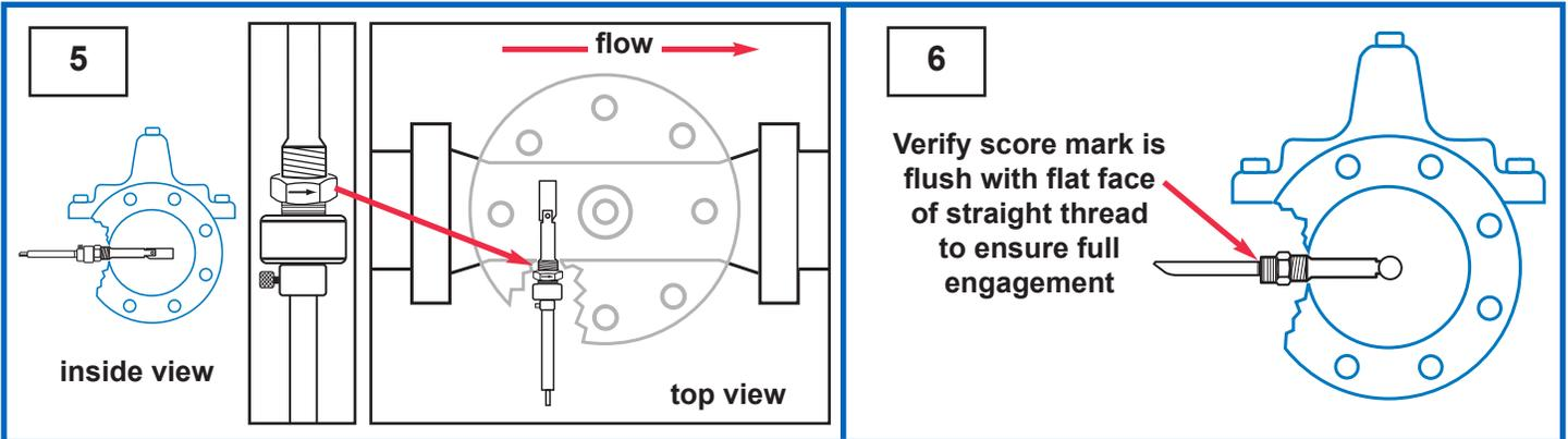
**Step 5:** Insert straightened Swivel Insert/Measurement Cylinder Assembly into valve, orient arrow on wrench flat to point downstream
