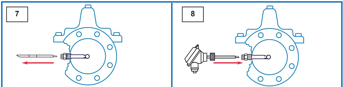
**Step 7:** Remove tool from Threaded Swivel Insert
