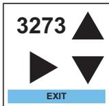
In this menu, a 20mA output signal is generated. To calibrate 20mA output to external device, use arrow keys to increase or decrease 20mA output. A Digital Multimeter to measure 20mA output. Select **EXIT** to return to Settings Menu.
