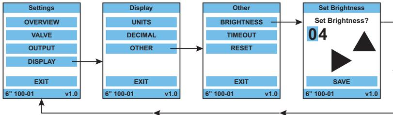
Use to increase/decrease screen brightness. Using a high setting will increase brightness, using a lower setting will reduce brightness. The default setting is 4. Use the right and up arrows to configure from 1 to 10.
