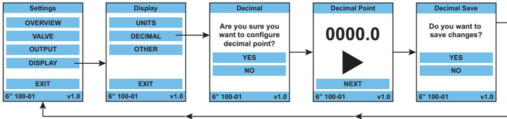
Flow decimal point may be set with up to two decimal places or no decimal point at all. Use the right arrow to configure decimal.
