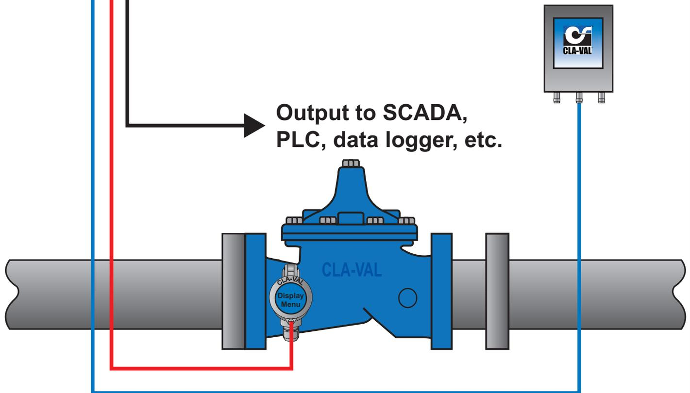
Combining additional Cla-Val electronic products with the X144D e-FlowMeter provides even more access to valve performance data installed in remote locations.
