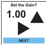
Default Gain is 1.00. Use arrow keys to adjust gain to desired value. Increasing or decreasing value offsets factory calibration. Select **NEXT** to continue.
