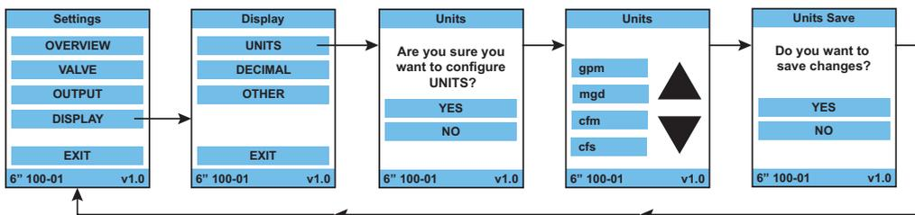
Use the up and down arrows to configure meter to appropriate units. When the correct units have been selected, 20mA scaling, pulse weight and flow cutoff values will update automatically. The following unit options are available, gpm, mgd, cfm, cfs, l/min, l/sec, m3/h, MI/d, and UK gpm.
