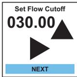
This setting is used to set a minimum flow reading that is displayed on screen before displaying zero flow. This is used when noise or vibration is causing erratic low flow readings when there is no flow. Select **NEXT** to continue.
