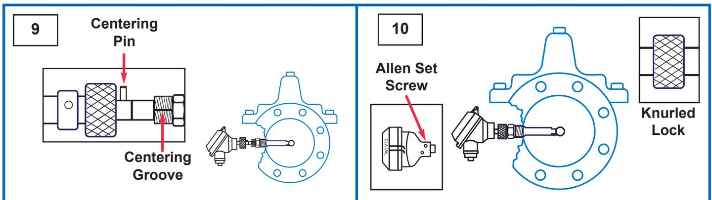
**Step 9:** Line-Up Centering Groove on straight threads with Centering Pin; push to seat o-ring
