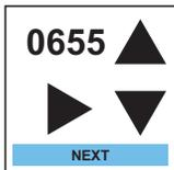
In this menu, a 4mA output signal is generated. To calibrate 4mA output to external device, use arrow keys to increase or decrease 4mA output. A Digital Multimeter to measure 4mA output.
