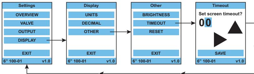
Use to configure when the LCD screen goes into sleep mode. Using a value of 00 will prompt the screen to always remain on. Use the right and up arrows to configure between 0 to 10 minutes, in one minute increments.
