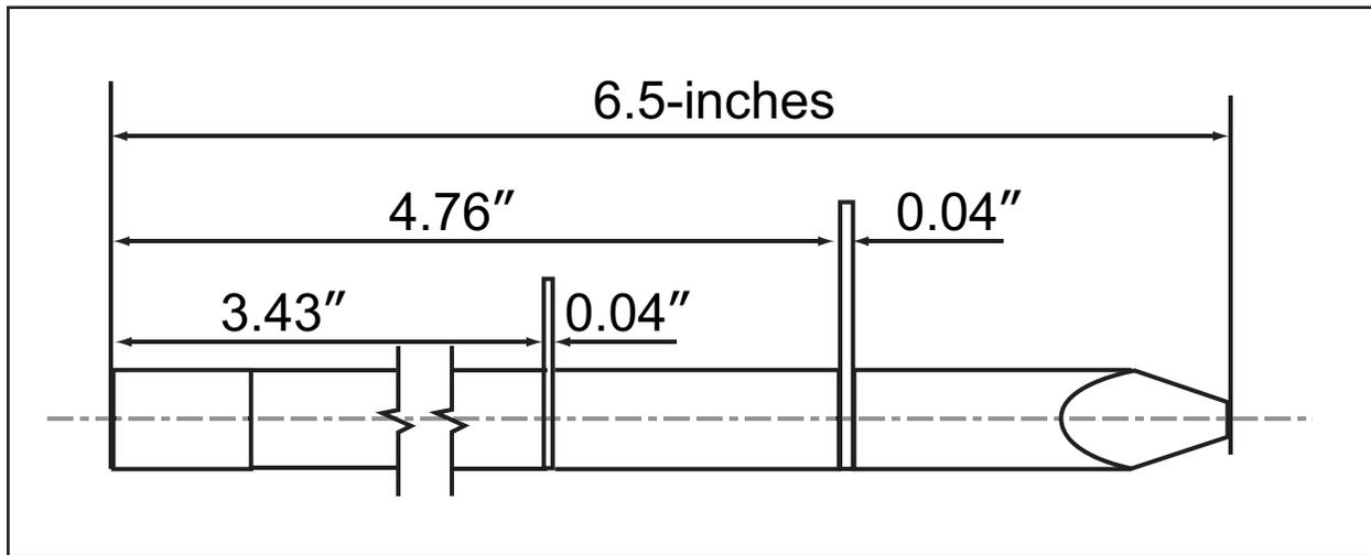
Figure 5-3: X144D Insertion Tool -  $T_2$
