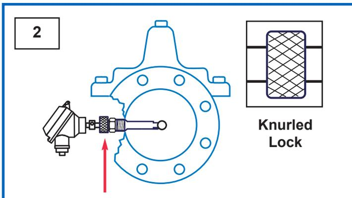
**Step 2:** After isolating the valve, bleeding pressure and disconnecting electronic devices, hand loosen the Knurled Lock from straight threads
