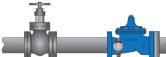
Install Isolation Valve (any style) a minimum of 5 pipe diameters upstream of the control valve
