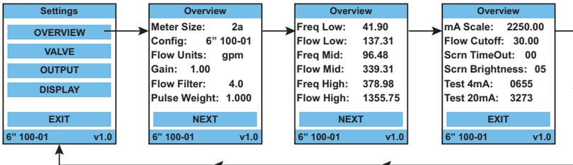
Displays all current parameters, useful when verifying parameters during commissioning. The overview menus display meter size, valve configuration, flow units, gain, flow filter, pulse weight, mA scaling, flow cutoff, screen timeout, screen brightness, and valve calibration.
