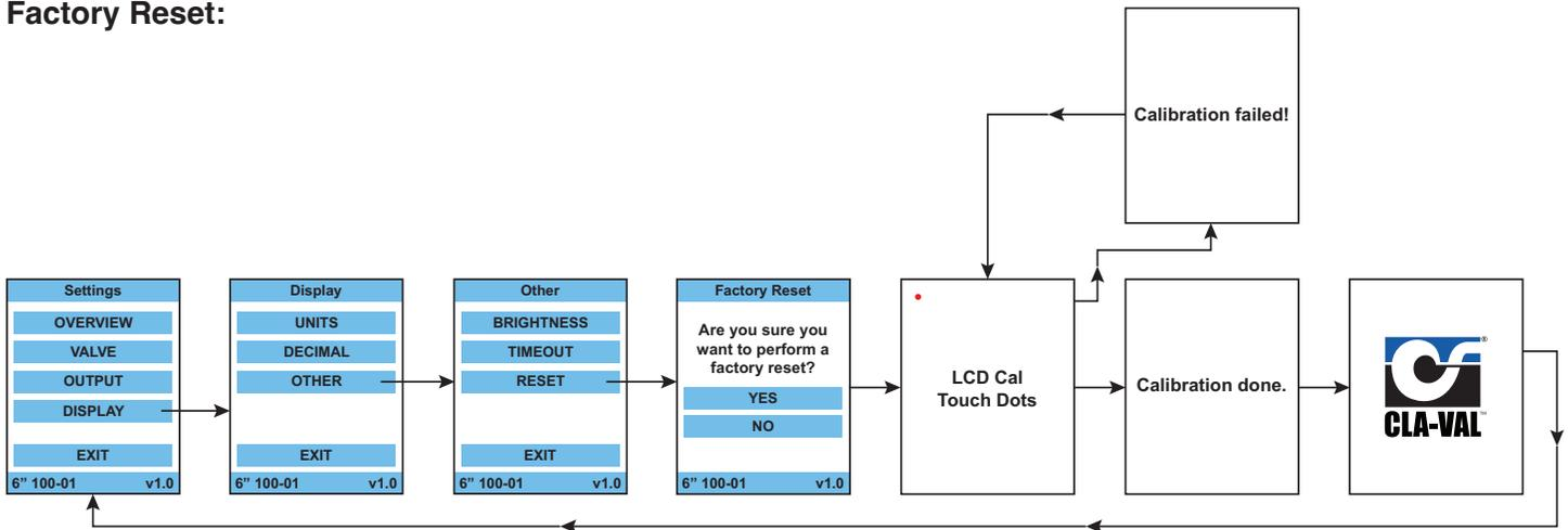
When a factory reset is selected, the LCD screen calibration will be reset and will prompt for recalibration. This should only be done if experiencing touch issues with the screen.
