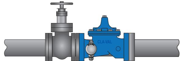
For installation directly onto the inlet flange of the control valve or where less than 5 pipe diameters upstream is the only option, an Isolation Valve **MUST** be a full ported, wide open Gate or Sluice style valve. In this scenario, the Isolation Valve **MUST NOT** be a Butterfly style valve.
