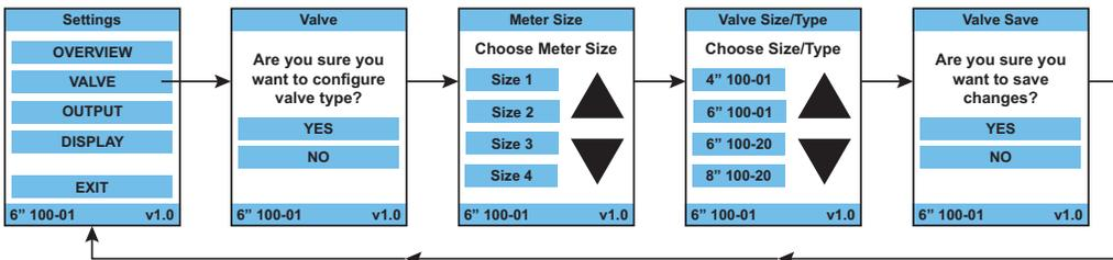
Follow onscreen menu instructions to configure meter size, valve size and valve type. First, select appropriate size meter; size 1, size 2a, size 3, or size 4. Based on meter size selection, a list of valve sizes and type will appear; select valve size that meter is installed in. Once selected, default parameters will populate into the fields described below.
