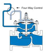
**Full Open Operation** When operating pressure below the diaphragm is applied and operating, pressure is relieved from the cover chamber and, the valve is held open, allowing full flow.
