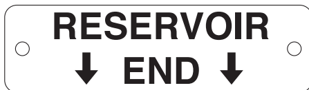
This brass plate appears on altitude valves only and is found on top of the outlet flange.
